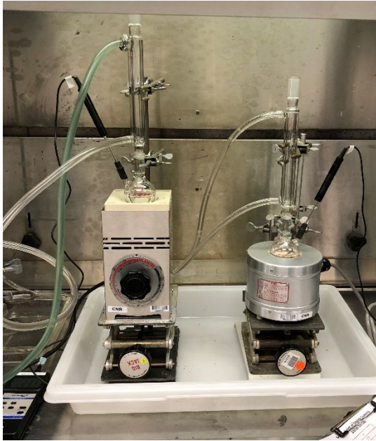
Figure 1. Test apparatus for ASTM D1120-17 ERBP. Heaters: Ful-Kontrol 750W (left), and Glas-Col 230W (right) Thermocouples: VWR Traceable RTD Platinum
